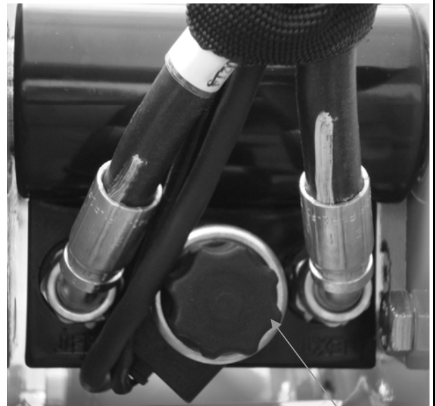
Figure 5-7. Cylinder Valve Removal
